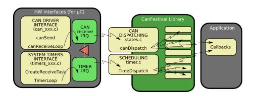
2. OS must provide a receive thread, a timer thread and a mutex. CAN reception should be a bloking operation.
