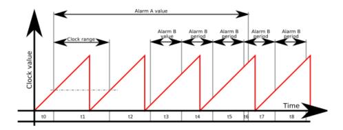
Scheduler can handle short clock value ranges limitation found on some  $\mu$ C. As an example, value range for a 16bit clock counter with 4 $\mu$ s tick is crossed within 0.26 seconds... Long alarms must be segmented.
