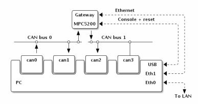
Figure 3.2: Testbed configuration.
