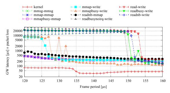
Figure 4.4: Latency and packet loss depending on the frame rate. Measured on MPC5200. The latency is the median of 3 200 measurements. Packet loss is drawn as error bars. For the sake of readability, error bars are magnified ten times.
