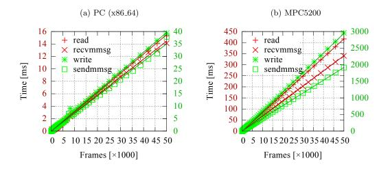
Figure 4.1: Comparison of read()/write() and recvmmsg()/sendmmsg() performance on a virtual CAN (vcan) interface. The straight lines show linear fit of the measured data. Note that reception times correspond to the left axis and send times to the right one.
