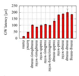
Figure 4.2: Latencies of various gateway implementations on MPC5200. A new frame was sent to the gateway only after receiving the previous one from the gateway. Bars show median, error bars span from the minimum value to 90<sup>th</sup> percentile.
