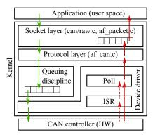
Figure 2.1: Linux networking stack architecture. Solid green arrows represent transmit data flow, red ones receive data flow. Dotted arrows represent notifications.
