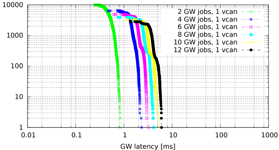
Chained GWs on a single VCAN interface (GW kernel 2.6.33.7-rt29-00004-g92487e4, Traffic flood, Load none)
