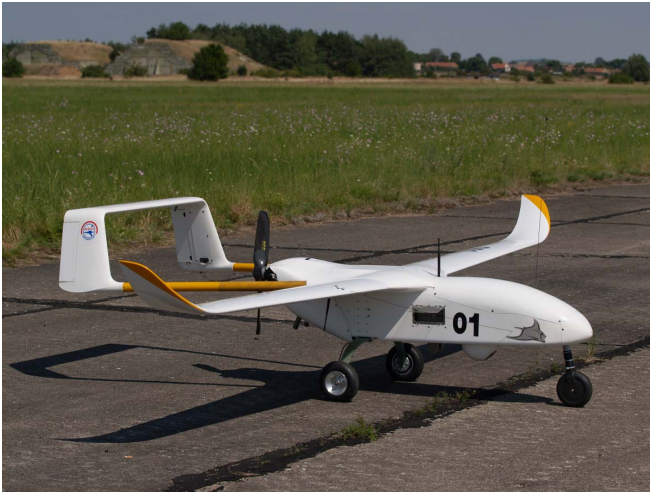
Fig. 1. Manta UAV - takeoff mass 58 kg, wingspan 4 m
