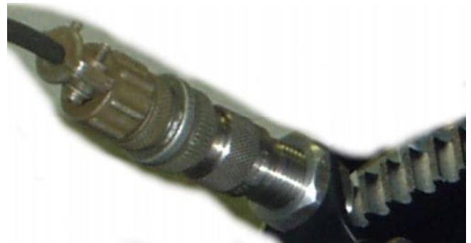
Fig. 5. Honeywell 3030 VRS RPM sensor measuring the main rotor RPM
