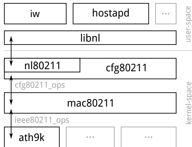
Figure 3.1.: IEEE 802.11 Linux kernel implementation architecture
