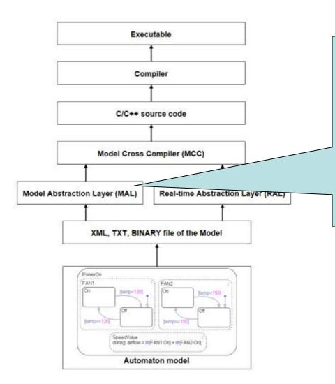
The purpose of the MAL (Model Abstraction Layer) is to create an independent interface between timed automata model and real-time entities (processes, threads, synchronizations, IPC) that will be automatically implemented. MAL is independent on the target HW and target operating system.
