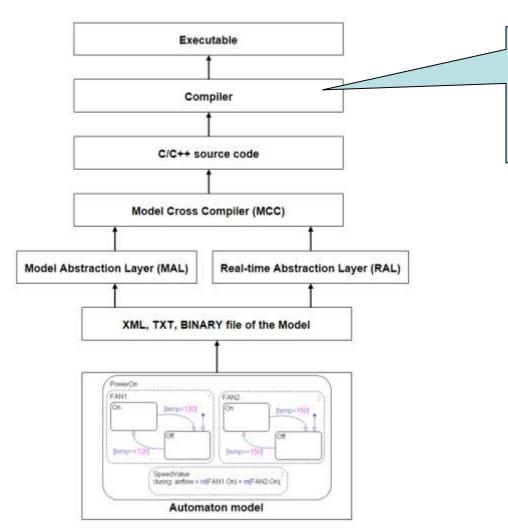
The source code can be included into the corresponding compiler and executable code for the target HW platform is generated.
