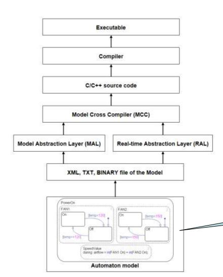
Formal model is created, simulated and verified using automaton diagrams.
