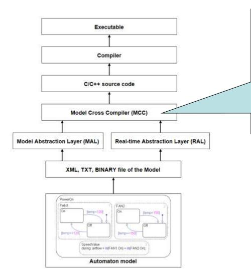
The Model Cross Compiler (MCC) is an interface for MAL and RAL transferring formal model of the system from the description tool into C/C++ source code.
