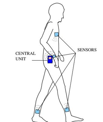
Obrázek 1: Principal spatial arrangement of the network nodes
