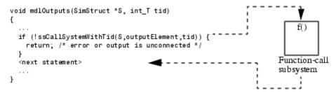
In this figure, ssCallSystemWithTid executes the function-call subsystem that is connected to the first output port element. ssCallSystemWithTid returns 0 if an error occurs while executing the function-call subsystem or if
