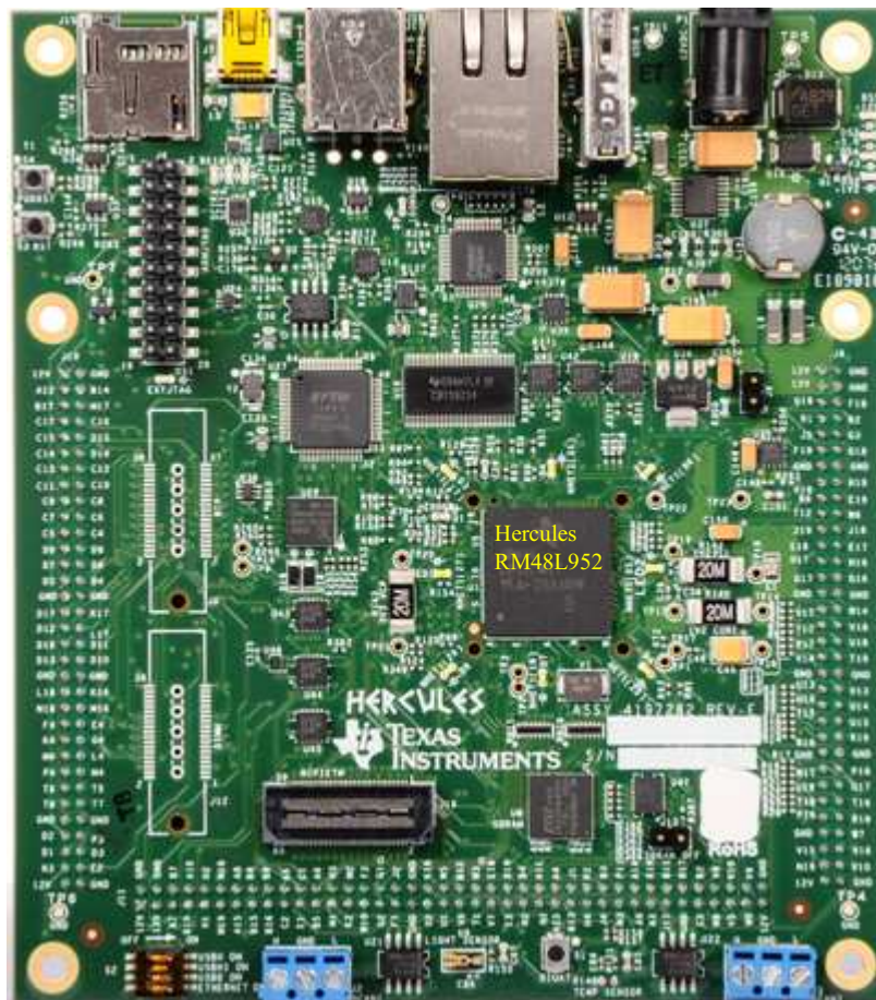
Figure 2-1. RM48 HDK Board, Interfaces Top Side
