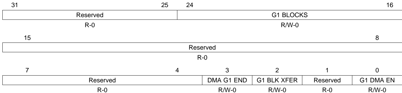
Figure 19-37. ADC Group1 DMA Control Register (ADG1DMACR) [offset = 50h]
