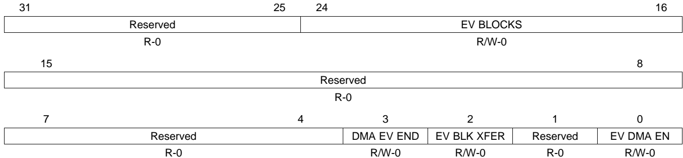
Figure 19-36. ADC Event Group DMA Control Register (ADEVDMACR) [offset = 4Ch]
