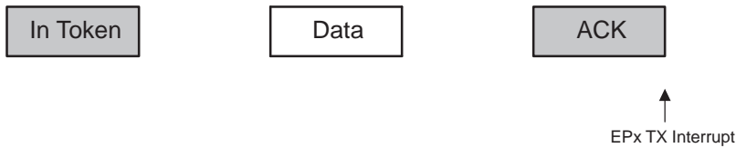
Figure 29-52. Non-Isochronous IN Transaction Phases and Interrupts
