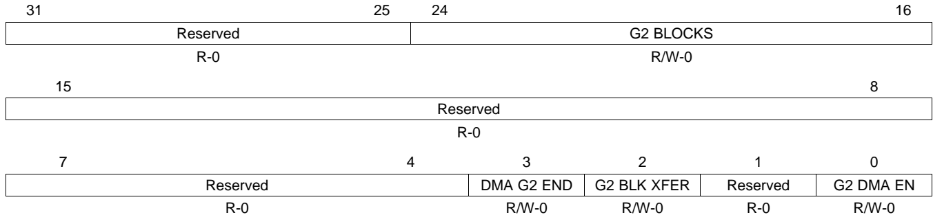
Figure 19-38. ADC Group2 DMA Control Register (ADG2DMACR) [offset = 54h]
