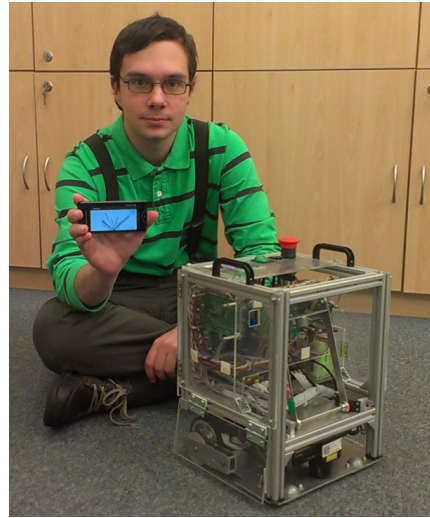
Figure 2: Controlling the robot with an Android phone.
