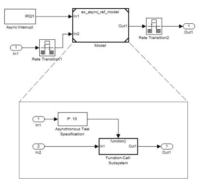
The Asynchronous Task Specification block must immediately follow the Inport block. Also, a branch cannot emanate from the signal connecting the Inport block to the Asynchronous Task Specification block.
