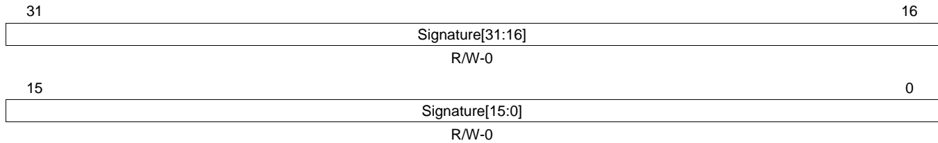
Figure 32-6. EFC Self Test Cycles Register (EFCSTSIG) [offset = 4Ch]
