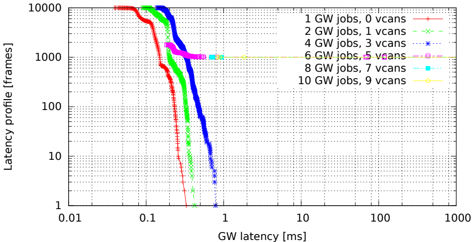
Chained GWs on multiple VCAN interfaces (GW kernel 3.0.4-rt14-00008-gb2052fd, Traffic 50, Load cpu)
