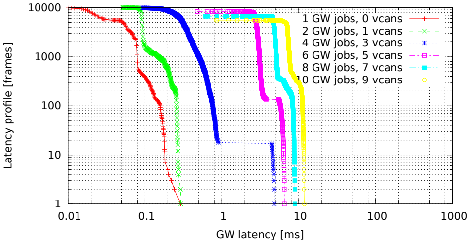
Chained GWs on multiple VCAN interfaces (GW kernel 2.6.36.2-00015-g4f1bc4e, Traffic flood, Load cpu)
